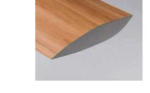
EGGER Laminate Micro is a decorative laminate based on curable resins. The laminate is constructed by fusing multiple layers and consists of melamine resin impregnated decor paper and a bondable reverse. Depending on application and requirements, the decorative side can be enhanced with a special overlay to increase surface abrasion resistance.
