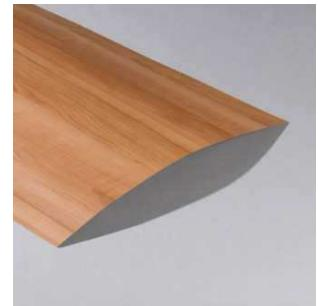
EGGER Laminate Micro is a decorative laminate based on curable resins. The laminate is constructed by fusing multiple layers and consists of melamine resin impregnated decor paper and a bondable reverse. Depending on application and requirements, the decorative side can be enhanced with a special overlay to increase surface abrasion resistance.
